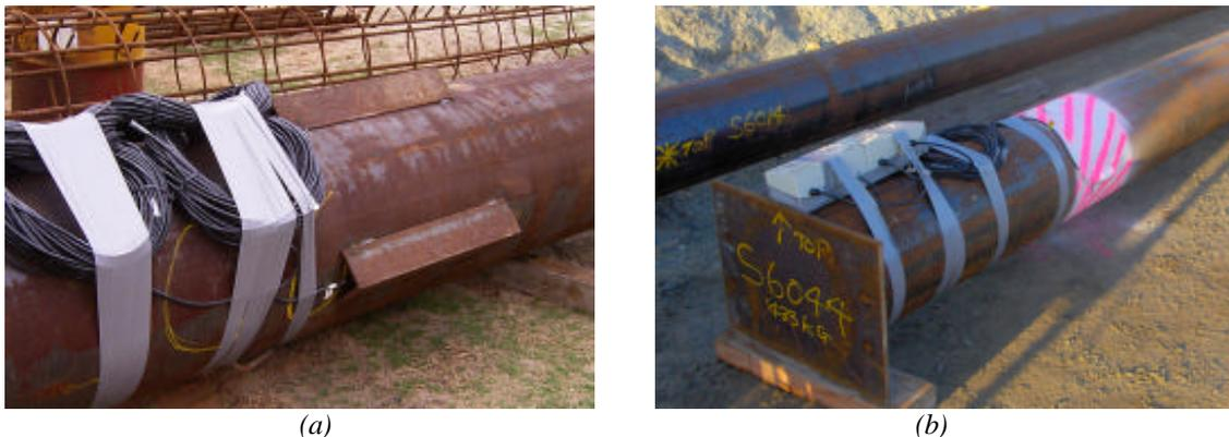
Figure 8. Instrumented strut with gauges protected by (a) welded angle section and where it was not possible to protect with welded section, (b) painted in fluorescent spray paint
