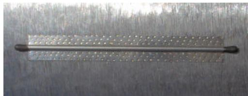
Figure 4 Spot welded strain gauge affixed to strut
